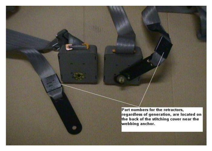
Part numbers for ALL retractors in the vehicle will be located on the black plastic stitching cover located near the webbing anchor.
