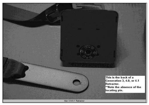
This is the back side of a generation 3, 4.0, or 4.1 retractor. Note the absence of the locating pin. Both mid-chair retractors mount with a 12mm x 25mm hex bolt, the sofa retractors mount with a 7/16"-20 hex bolt.
