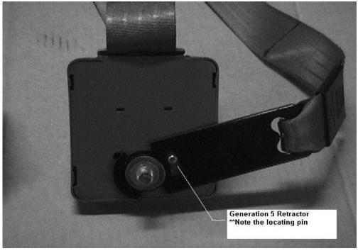
This is the back side of a generation 5 retractor, which is currently in use. This series of retractors are different in a couple of ways, one is that they now have a pin to locate the correct angle, and two, they have a  $\frac{1}{2}$ "-13 stud in place for the sofa retractors (see above photo). The mid-chair retractors do not have a stud, but will install in the usual way.
