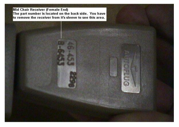
Mid-chair receivers' part numbers are located on the back side of the receiver. For this part, you'll have to remove it from the seat pedestal/seat slide and pull it out of it's plastic sleeve to view the part number. Please write down all numbers on the part and note the color.
